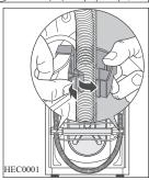
**3.** With the provided spanner unscrew and remove the central rear bolt **A.**
